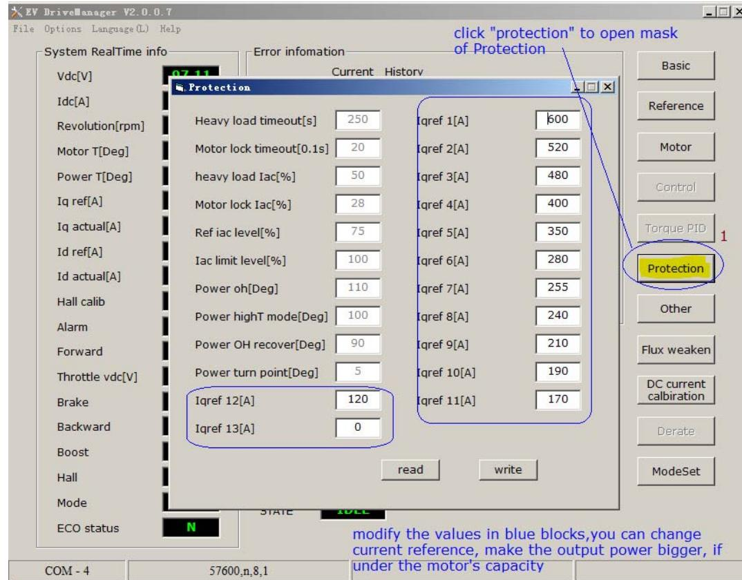
with the former method, If you still can't reach the speed you wanted as 130kph, about 1146rpm of motor speed. you can
